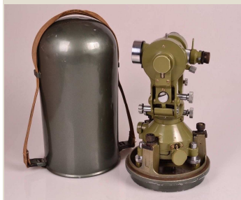
Figura 1.8 – Teodolito Wild T2. Fonte: https://www.ebay.com/itm/Excellent-Wild-T2-Theodolite-Heerbrugg-Switzerland-S-N-101188-Free-Shipping-/302643108242
