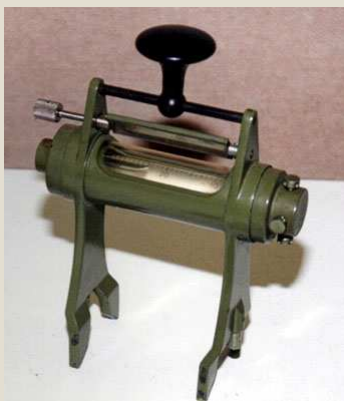
Figura 1.10 – Nível de cavalete. Fonte: http://www.sage.unsw.edu.au/currentstudents/ug/projects/f_pall/html/t29.html
